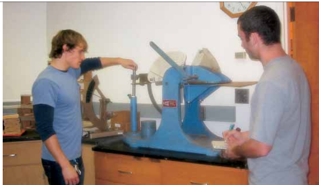
Students Braden White and Jim Bisha perform TMI puncture tests on corrugated packaging.
